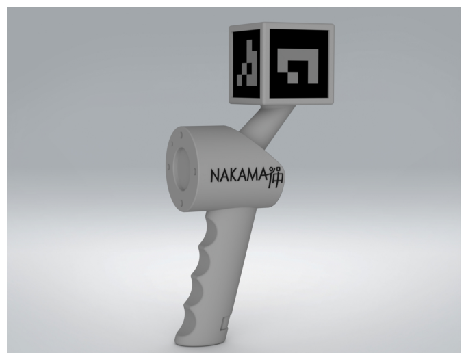
Figure (1) The designed modular handheld proxy device for LfD, with an ArUco marker cube, a flange designed for robotics, internal cable routing, and a cable retainer to secure the cables of possible added sensors.
