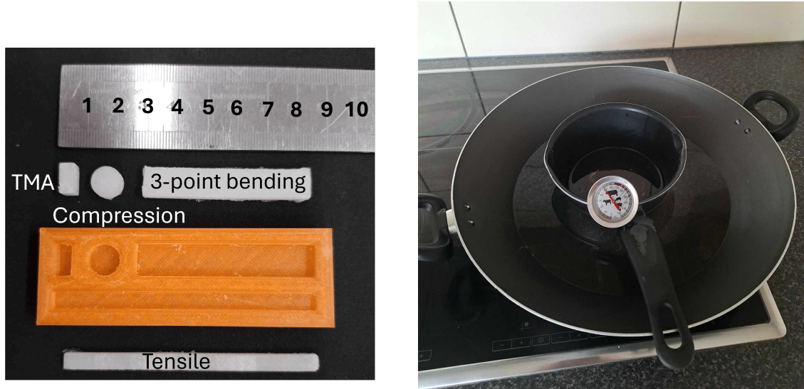
(a) 3D printed mould with the corresponding samples
