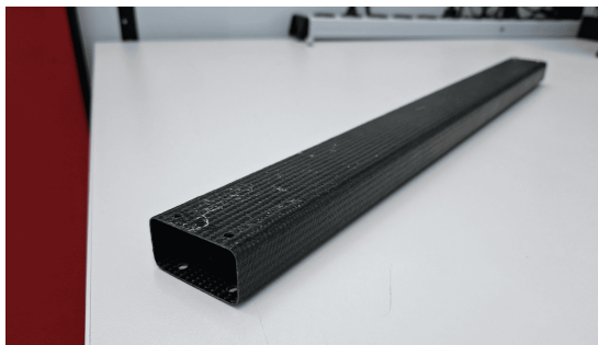
(a) Close up of the outside of the beam. Shown are the small holes to attach the plastic cap (top and bottom) and the weave pattern of the carbon fibre
