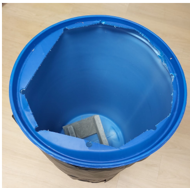
Figure 3.3: Barrel test setup into which other pipes were placed and the robot was lowered into from above.
