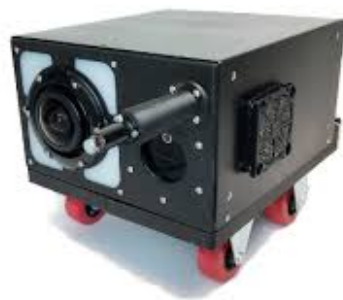
Figure 2.5: Wheeled cart with camera and LED [ 17 ].
