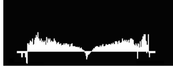
Figure 62: Resulting scoring histogram. The x-scale for the histograms is from edge value -128 to edge value 128 where the center edge value is zero. The y-scale indicates the chance of the value being on the limb, or in the background, where above zero is belonging to the limb, and below zero is belonging to the background.
