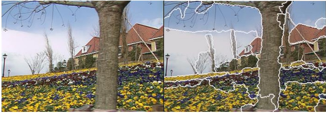
Figure 23: [DENG] Left: original input image. Right: segmented image using color and texture information.
