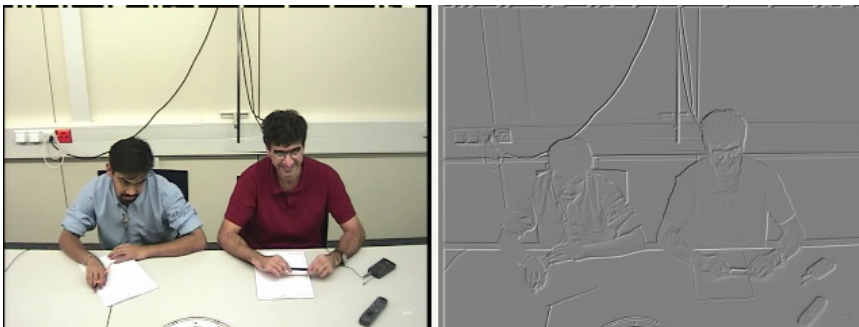
Figure 28: Left: original image. Right: edge image using Sobel kernel.
