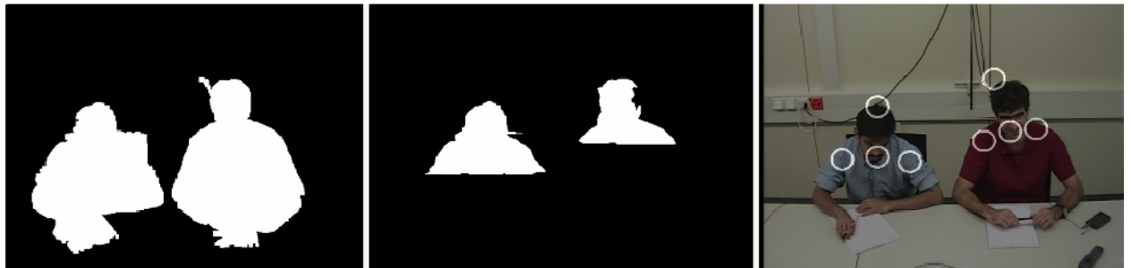
Figure 74: Left: input silhouette. Middle: resulting best match after snake. Right: resulting coordinates. The right silhouette matches with a different template, which has different coordinates. After one or two frames the system detects this error and will re-initialize the template.
