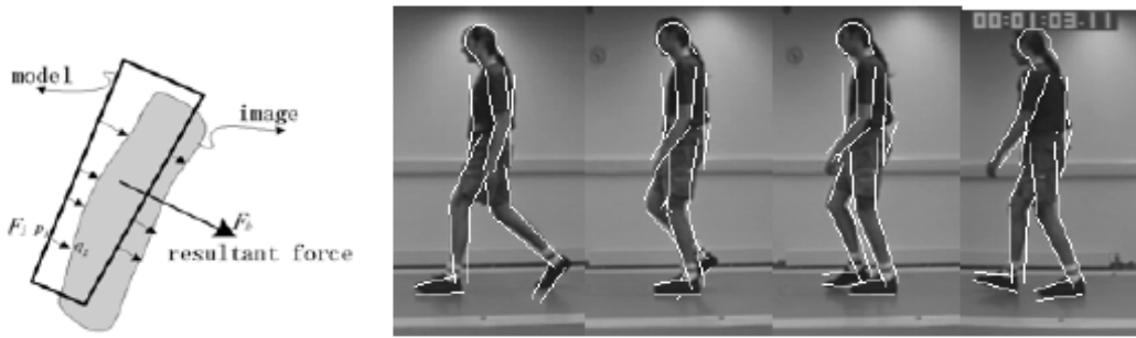
Figure 36: [NING] Using optical flow to align a body model with the actual image.
