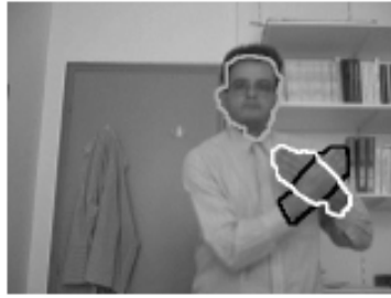
Figure 26: [ARGY] Using skin detection to detect head and hands.
