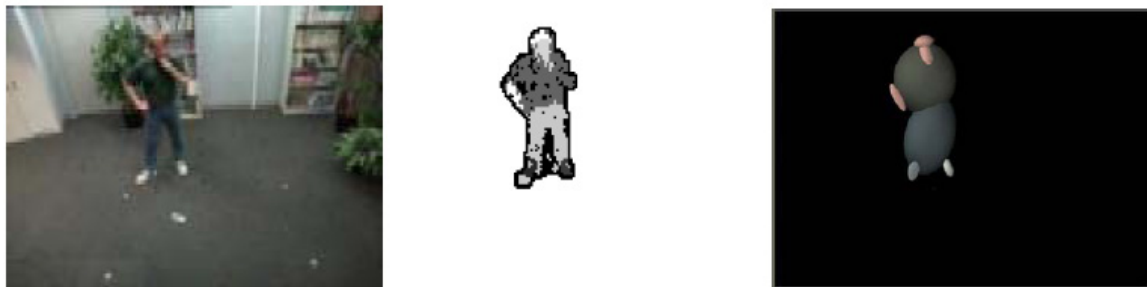
Figure 21: [WREN] Left: original input image. Middle: color segmentation into blobs. Right: 3D-blob representation of the person.
