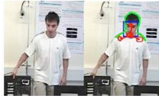
Figure 16, [LEE], left: original input image, right: detected contour and shoulder points are displayed.
