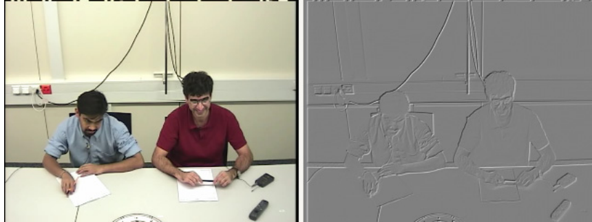
Figure 40: Left: original image. Right: edge image using Sobel kernel
