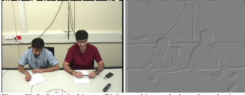
Figure 59: Left: original image. Right: resulting angle dependent edge image.
