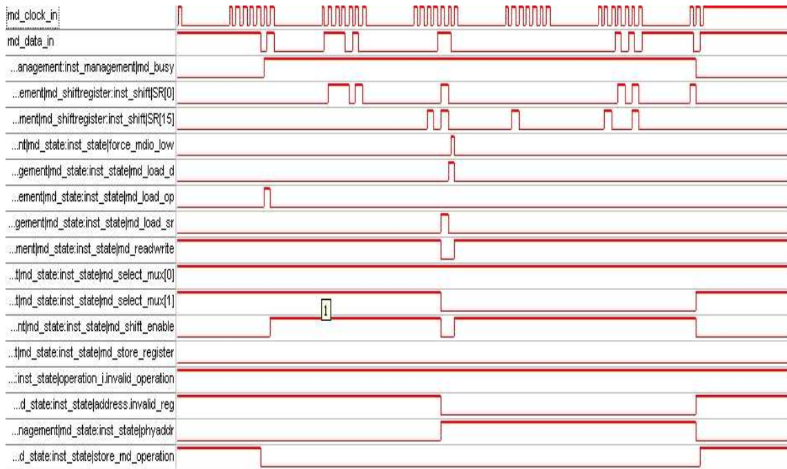
Figure 6.5: MII read frame inside FPGA
