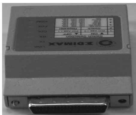
Figure 3.3: The Edimax MII transceiver
