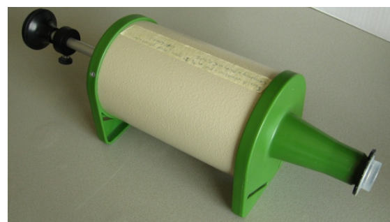
Figure 8-7: manual artificial lung. Prototypes can be connected on the right side. Moving the black handle on the left mimics breathing.
