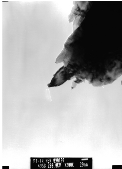
Figure 2.5: A transmission electron microscope image of an scanning tunnelling microscope tip [22].
