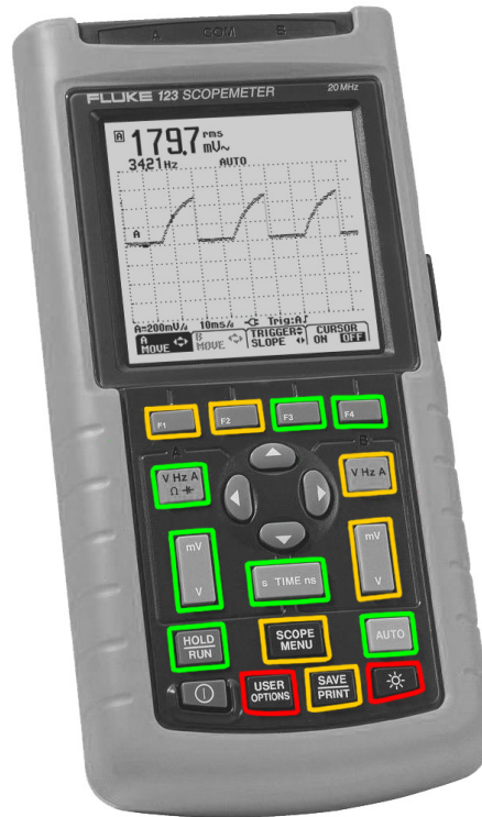
Figure 14: keypad marked according to importance of the corresponding function or menu
