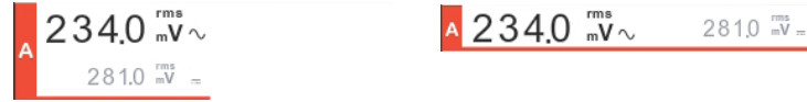
Figure 89: reading area with one signal in the original concept (left) and the redesign (right)
