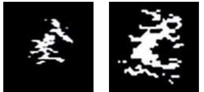
Figure 9: Deformation of the ultrasound images during the experiment caused by air in the target, non-conducting chicken breast tissue or needle placement above the target.
