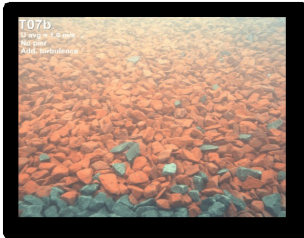
Figure 3-4: One frame of the video of camera 1. Camera 1 filmed the condition uniform flow and the condition sill-induced additional turbulence. The flow direction is from left to right.
