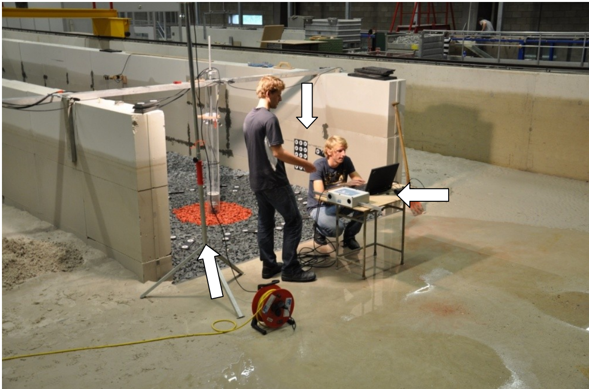
Figure 3-7: Stereo photography set. The set contains the camera attached to a laptop (on the table), the markers (around pile) and baseplate (attached to wall).
