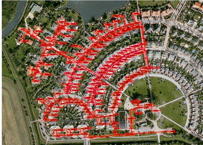
Figure 3.2: The structure of the cables in Lochem projected on a satellite image from Google maps. (source: [24])
