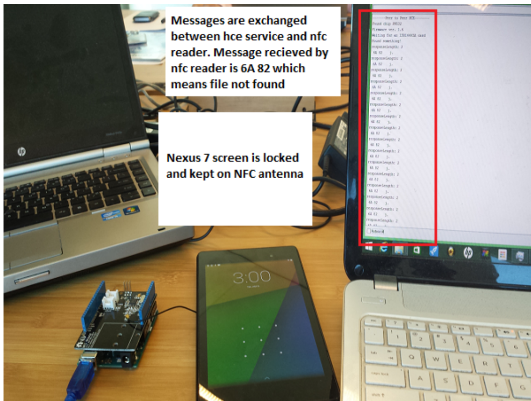
Figure 7.15: Google Wallet communicates with the NFC reader when the device is locked
