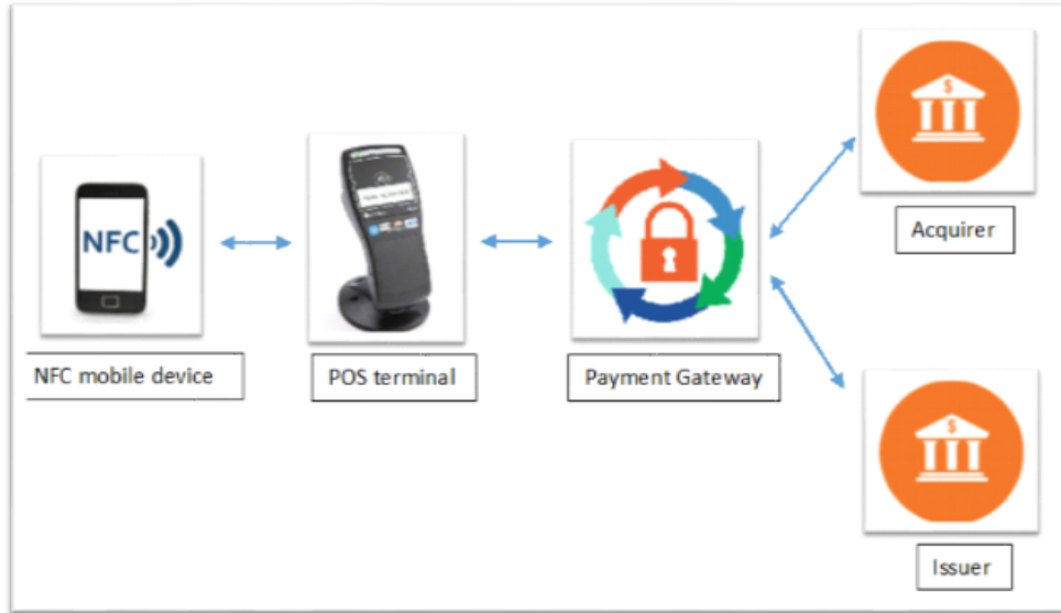
Figure 2.2: The transaction flow and key parties in mobile payment model. Adapted from [15]
