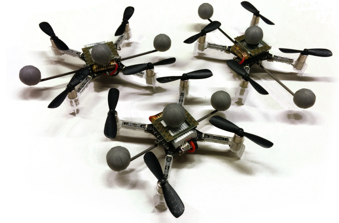
Fig. 19. Photograph of the Crazyflie 2.0 that are used.
