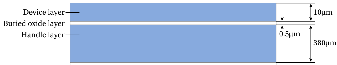
Figure 2.11: Schematic representation of SOI wafer with dimensions
