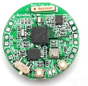
Figure 2.1: RealTag CC2541 sensor with accelerometer, pressure sensor and Bluetooth low energy transmitter. This compact sensor has the size of a 2-euro coin and is powered by a small battery on the back.
