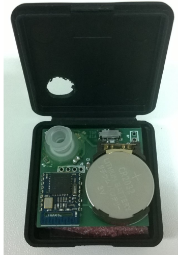
Figure 2.2: Our custom made printed circuit board containing an on/off switch, pressure sensor, accelerometer and Bluetooth transmitter. On the left top, a white connector for a nasal cannula is shown with the pressure/temperature sensor underneath. The left bottom shows the Bluetooth board. Below this board the accelerometer is positioned. This first design used a CR2032 battery. The box size is 40 x 40 x 20 mm (L x W x H).
