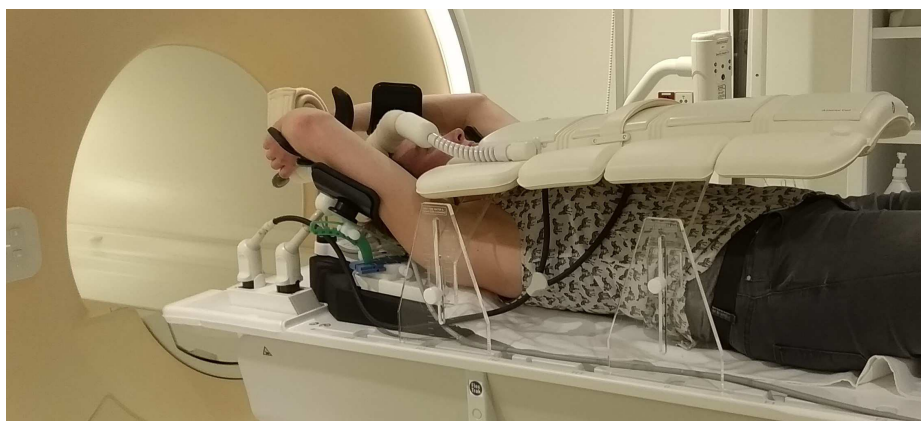
Figure 2.1: MRI scanning set-up with flat table top, TAS, coil bridges and receive coils.
