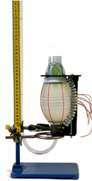
Fig. 3: Test setup with a ventilation balloon as a heart model.
