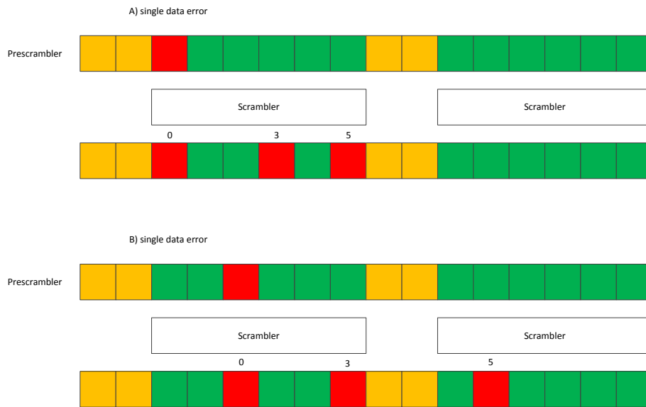
Figure 12 Error propagation to the next word. In A the error stays within one word; in B it crosses the word boundary.
