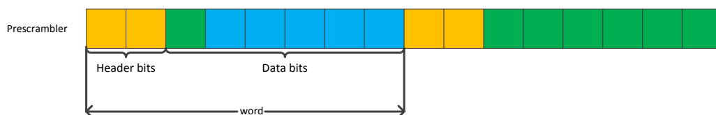
Figure 11 Blue bits are errors that propagate to the next word
