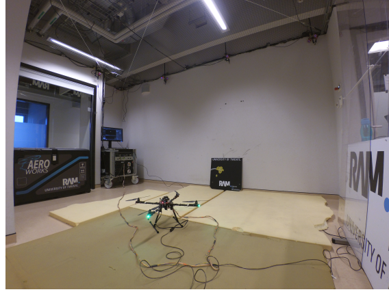
Figure 6.11: Picture of the experiment setup. A power cable and usb cable are connected to the quadrotor. The computer visible on the mid-left of the figure runs the OptiTrack software and publishes the measured odometry over a wired network connection to an external laptop running ROS. The usb cable is also connected to the laptop running ROS to establish MAVLINK communication with the Pixhawk.
