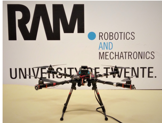
Figure 6.9: Quadrotor used during the experiments. The cable visible in the figure is the MAVLINK USB-interface and is connected between the Pixhawk and the laptop running ROS. During experiments, an additional cable was connected to the quadrotor to provide power, such that no onboard battery was needed.
