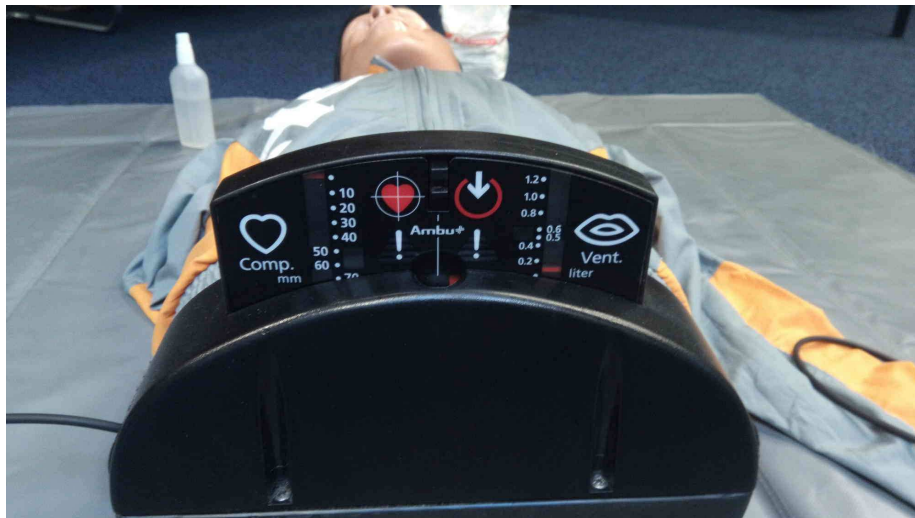
Figure 2.2: CPR doll used at a course, gives basic feedback to surrounding students about compression depth (left), hand position (middle) and volume of breath (right).
