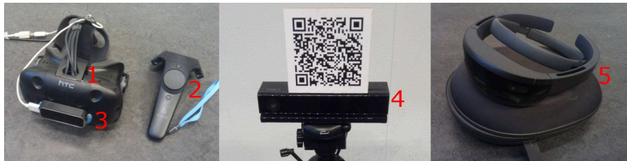
Figure 4.1: Hardware used: 1. HTC Vive headset; 2. HTC Vive controller; 3. Leap Motion mounted on headset; 4. Kinect for Xbox One with a QR code to determine the position; 5. Hololens.
