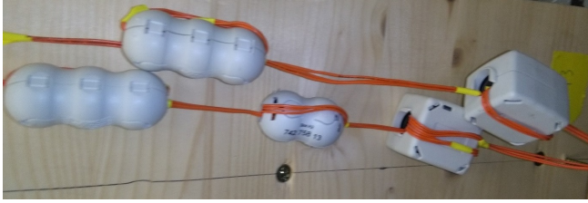
Fig. 8. Ferrite clamp-on cores wrapped around the wires between the sensor and microcontroller.
