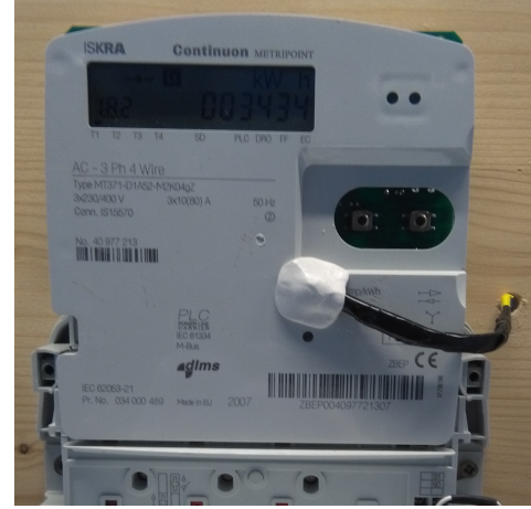
Fig. 5. Optical sensors as attached to a static meter
