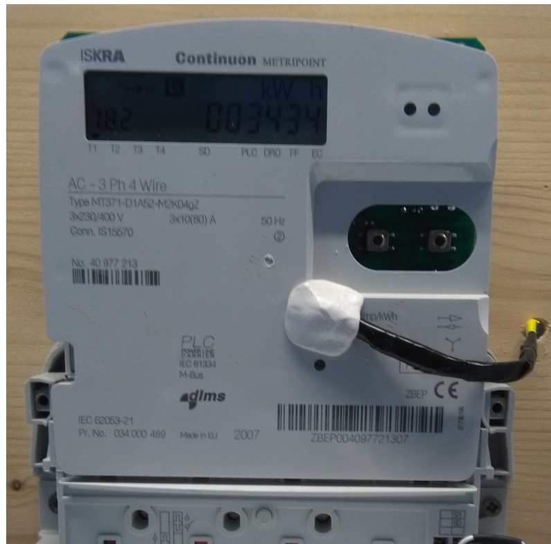
Figure 3.1: Optical sensor attached to a static meter.
