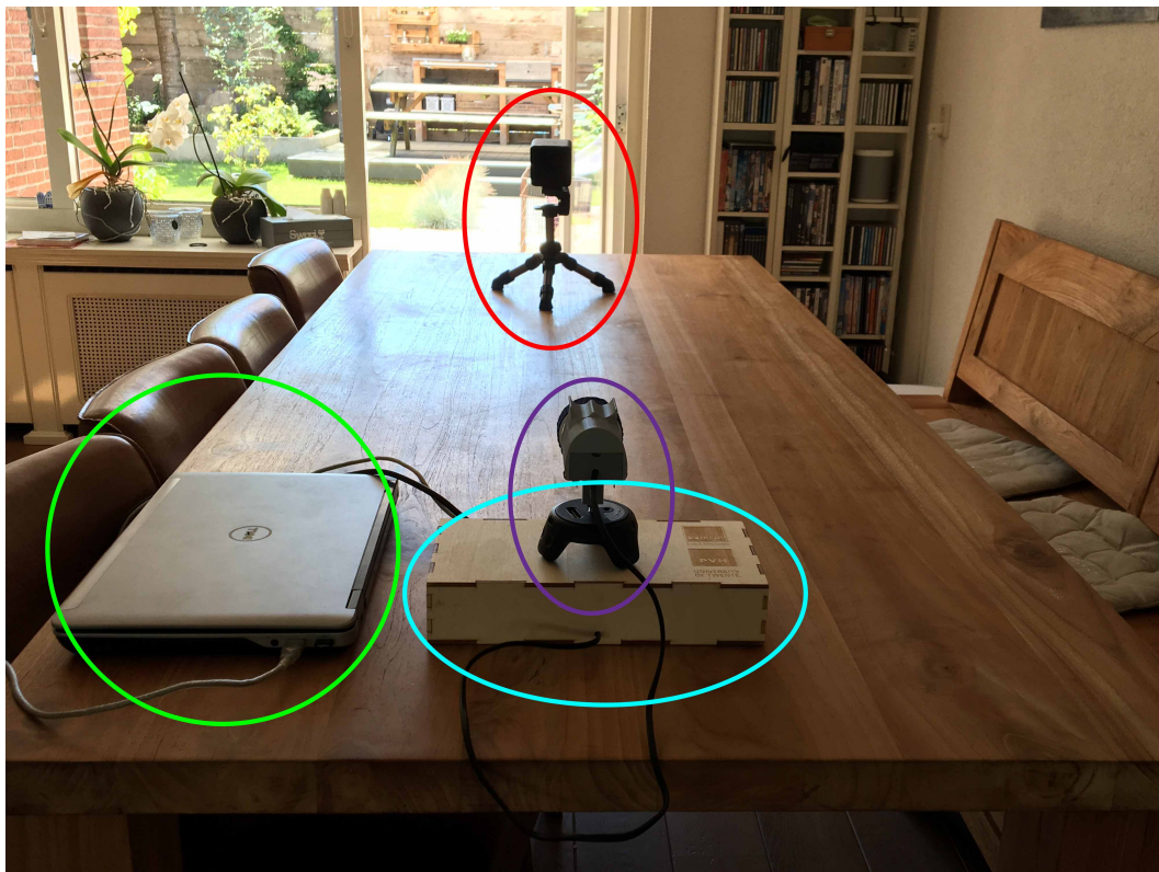
Figure 21 – Set-up of the prototype with the controller including a haptic wheel (inside purple circle), the box with electronics (inside blue circle), a laptop (inside green circle) and the HTC VIVE tracking system (inside red circle).
