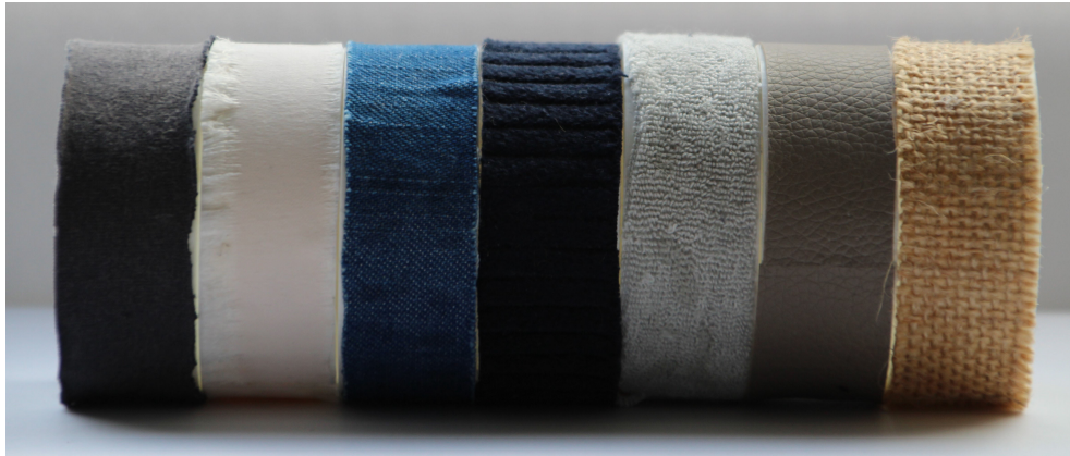
Figure 23 – The seven haptic wheels, each with a different fabric attached on top. From left to right: Cotton, Satin, Denim, Rib fabric, Terry, Leather, Sackcloth.
