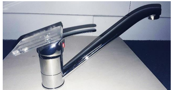
Figure 33: Side view of the sensor attachment piece on the faucet
