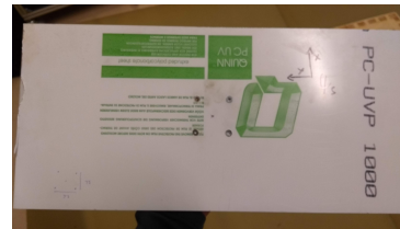
(b) Interaction plate which is mounted on top of the torque sensor
