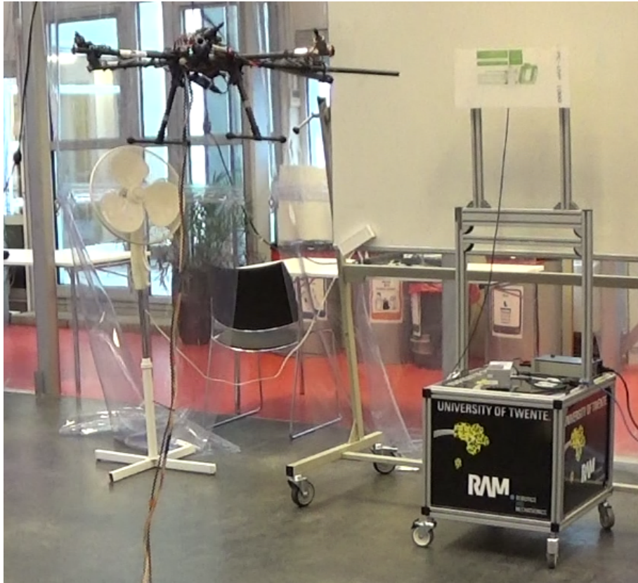
Figure 5.5: A picture of the experiments which includes sources of disturbances
