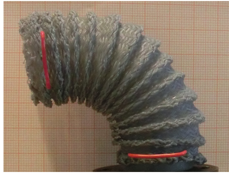
Figure 1.1: MOLLUSC module bending (Jansen, 2018)
