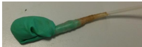
Figure A.1: The granular jamming sac used for stiffening the MOLLUSC design (Gifari, 2018)
