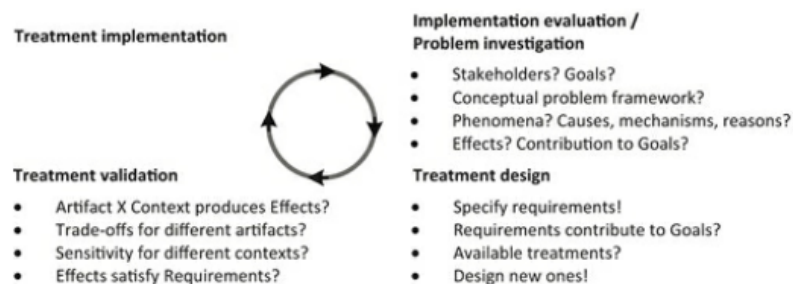
FIGURE 2.2: The Engineering Cycle ([75, Fig 3.1])
