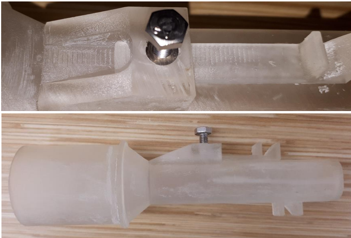
Figure 9 - Adjustable mouthpiece with a close-up of the measure lines.
