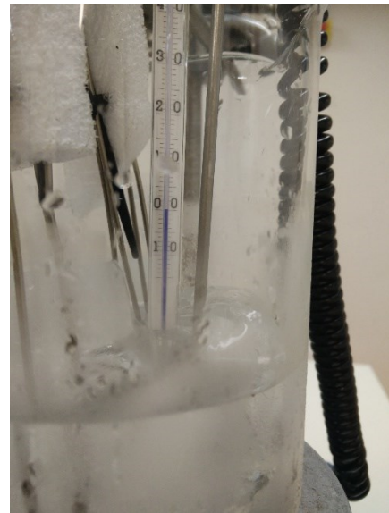
Figure A2.10: RTD calibration at 0°C.
