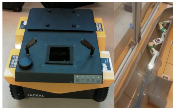
Figure 4.7: Real-World Experiment Robots available in RAM lab at University of Twente. Left image is of the Clearpath path differential drive mobile robot (Jackal). Right image shows PIRATE inside 125mm pipe.
