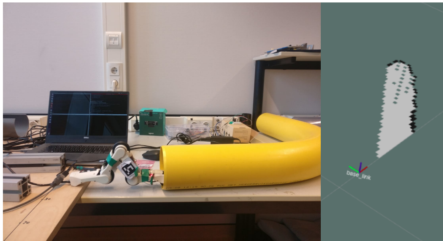
Figure 5.18: Testing of PIRATE in a curved pipe of diameter 120mm. The left image shows the environment set-up while the right images shows the construction of Occupancy grid map. It fails to produce the map since the LiDAR is unable to detect the surface of the pipe due to its minimum range.
