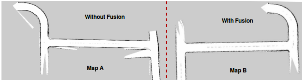
Figure 4.3: Pre-built map used for AMCL implementation. Map generated using Gmapping. Map A is created without sensor fusion and Map B is created using sensor fusion.
