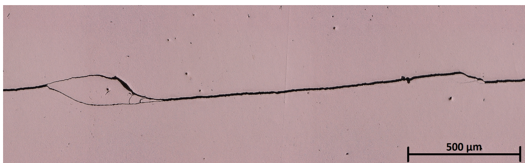
Figure 5.6: Split cracks in clamp region that showed up after polishing (sample 6903-3A)
