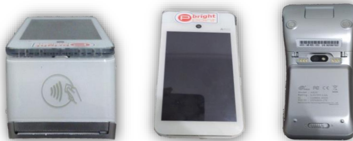
Figure 17. EDC (Left: NFC Reader, Magnetic Card Reader, and Printer, Middle: Screen, Credit Card Dip, and QR Scanner, Right: QR Scanner, Battery Inside, and Cellular Sim Connectivity Inside)
