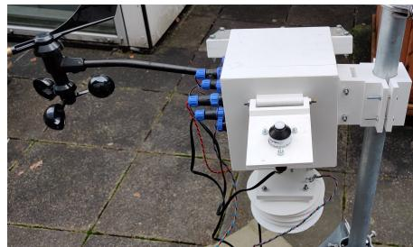
Figure 16: The assembled sensor node housing
