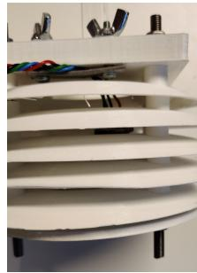
Figure 23: Picture of radiation shield
