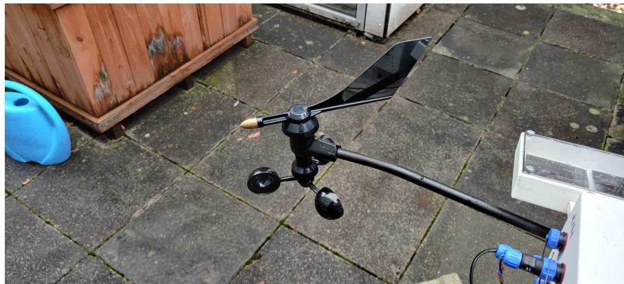
Figure 10: Anemometer from Davis Instruments
