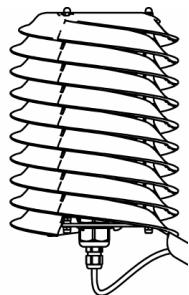
Figure 2: Helical design radiation shielding
