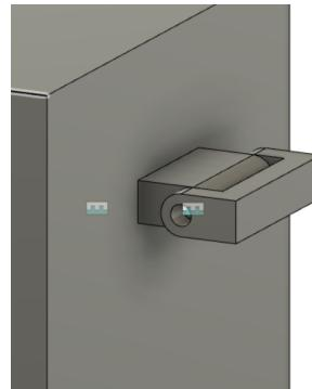
Figure 7: Hinge Sensor Connection
