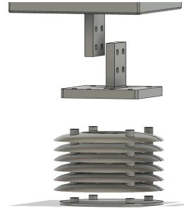
Figure 24: 3D model of solar radiation shield
