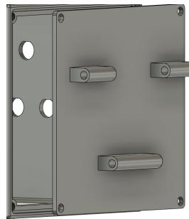
Figure 20: The lid of the sensor node
