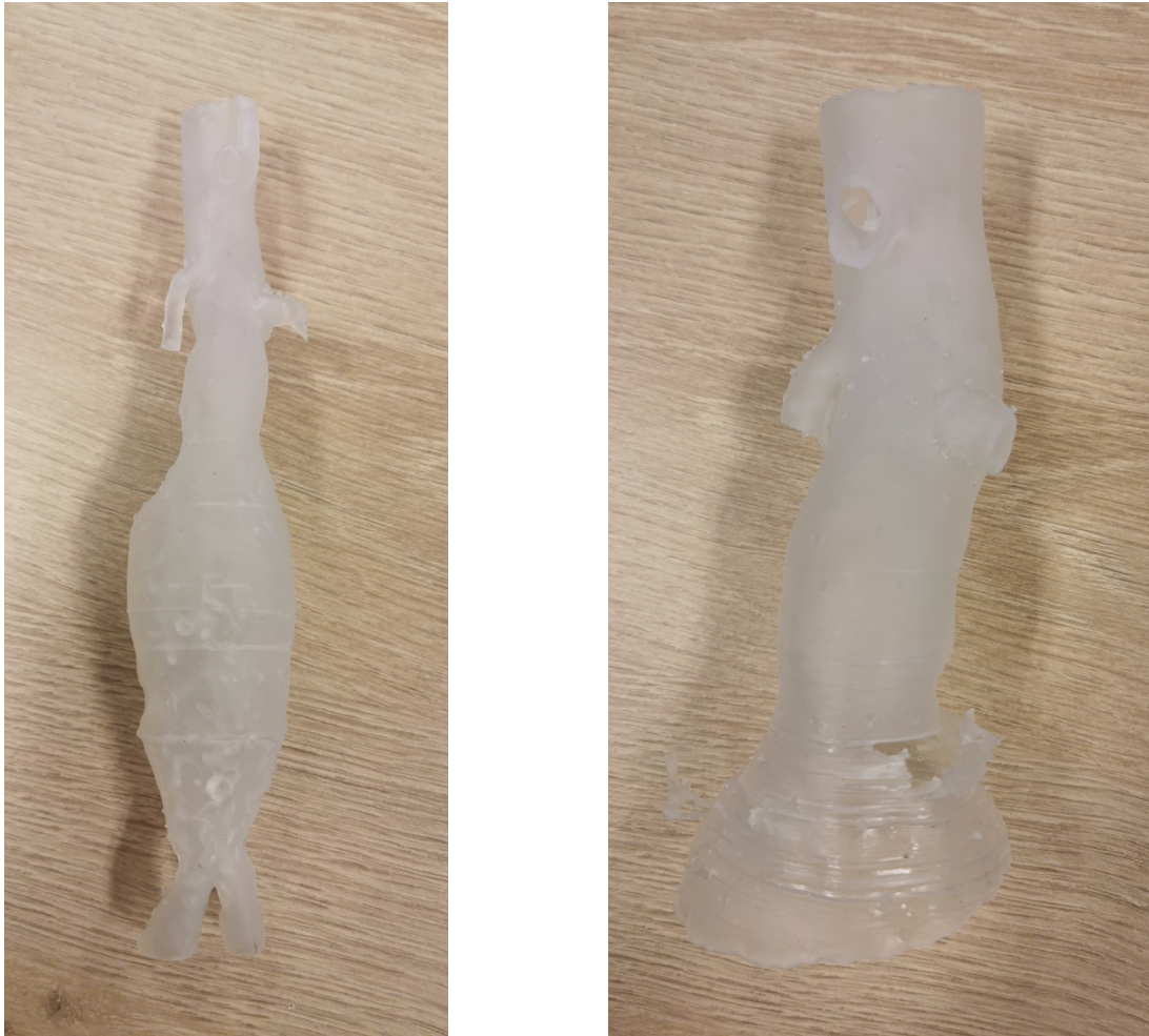
Figure 16: Aorta models printed in elastic resin. On the left, an aorta with the branches of the renal arteries, the complete aneurysm and bifurcation to the iliac arteries are shown. On the right, an upper part of the aorta and aneurysm can be seen, including the branches of the renal arteries and superior mesenteric artery. In the aortic neck and upper part of the aneurysm, tears are visible.
