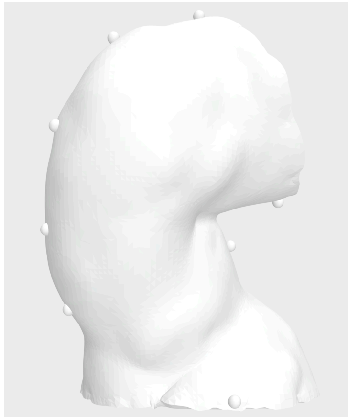
Figure 20: Aorta model with spheres. The displacement of the spheres is measured and this is used to calculate the distension of the aortic wall in the models when a stent graft is placed.
