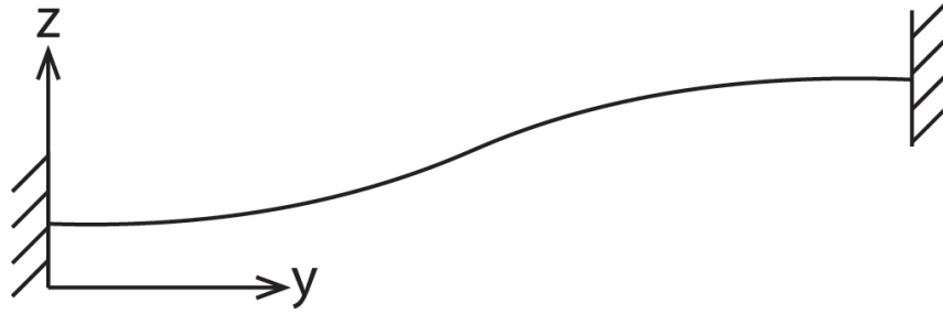
Figure 3.1: Bending shape for double clamped leaf spring.
