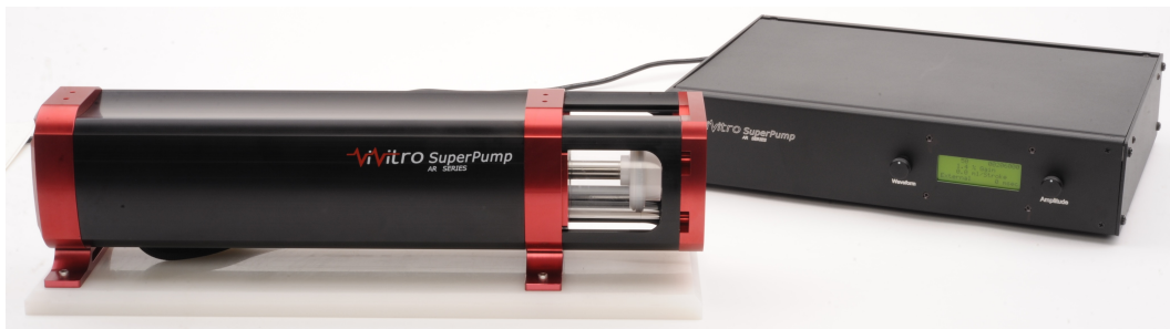
Figure 12: ViVitro SuperPump with a controllable piston, a fluid chamber and mechanical valves inside. The waveform and amplitude can be set by the controller. [24]
