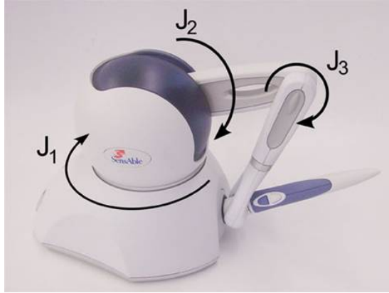
Figure 9: The PHANTOM Omni, with the three joints capable of providing force feedback labeled.
