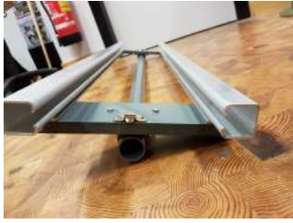
Figure 35: One meter piece with the rails installed and connected to each platform.
