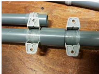
Figure 31: PVC tube with the platform holder glued to it
