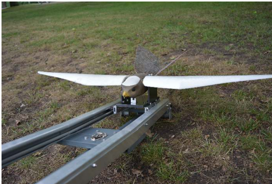
Figure 20: Robird on the cart ready to be launched
