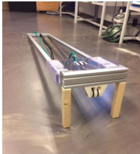
Figure 6: A bungee based Robird launching ramp developed by students
