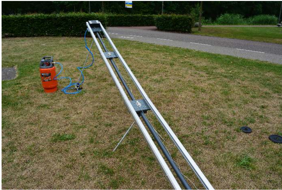
Figure 19: Complete pneumatic launching ramp, with a total weight of 23.840 including the air tank.
