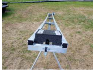
Figure 36: The damper and the pulley installed at the end of the ramp.
