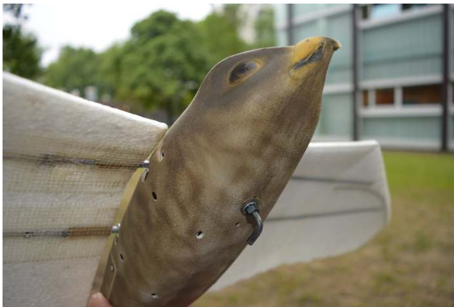
Figure 22: Hooking mechanism attached to the Robird.
