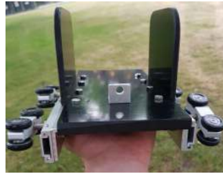
Figure 38: Complete cart with the hook and wheels.
