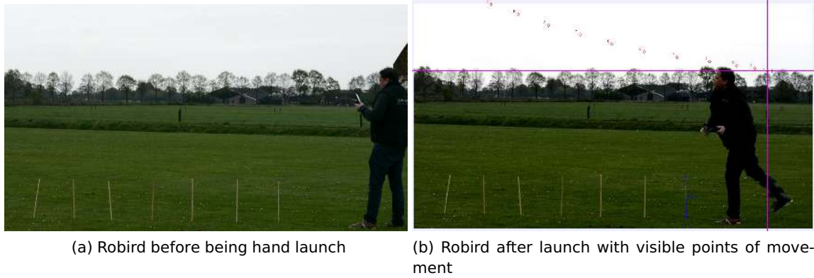
Figure 23: Measurement of the angle and velocity during hand launch
