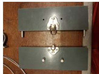
Figure 34: The clamps and pins are added to improve alignment
