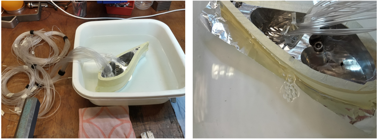
Figure 4.15: Checking airtightness of circuits: (l) Submerging measurement section in water. (r) Looking for bubbles appearing in water.
