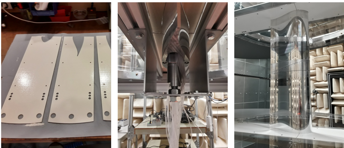
Figure 4.18: Wooden end-plates enclosing the wing in the test section (l). Installing the wing in the test section from below (m) and the wing suspended in the test section enclosed by the wooden end-plates (r).
