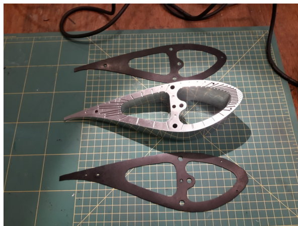
Figure 4.14: Assembly sealing surfaces: (l) Rubber gaskets cut to compensate unevenness. (r) Application of vacuum grease to fully seal the pressure circuits.
