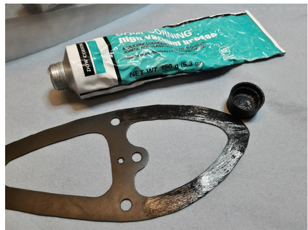
Figure 4.14: Assembly sealing surfaces: (l) Rubber gaskets cut to compensate unevenness. (r) Application of vacuum grease to fully seal the pressure circuits.
