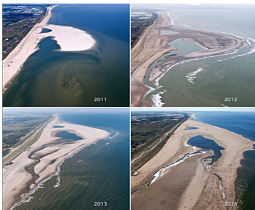
Figure 3 The Evolution of the Sand Motor since its Construction in 2011 Source: Dutchwatersector.com (2016)
