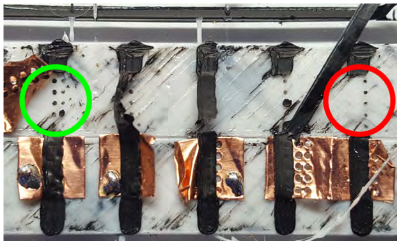
Figure 4.14: [NOTE: bed temperature 40°C] Here you can see that in the green circle the fusion was properly, you can clearly see more black dots than in the red circle, 1 row of dots is entirely missing.
