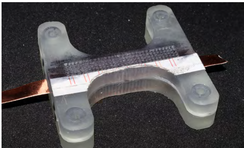
Figure 5.3: Special designed jig to punch 600 \mu\text{m} in a controlled way in the copper tape. the jig ensures a constant alignment of the tape and allows the user to punch 10 or 1 hole at the time. The 10 hole punch is not included in the photos.
