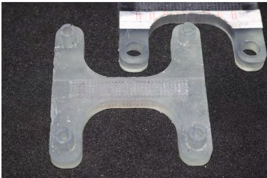
Figure A.6: Jig used to puncture holes in phase II in greater detail
