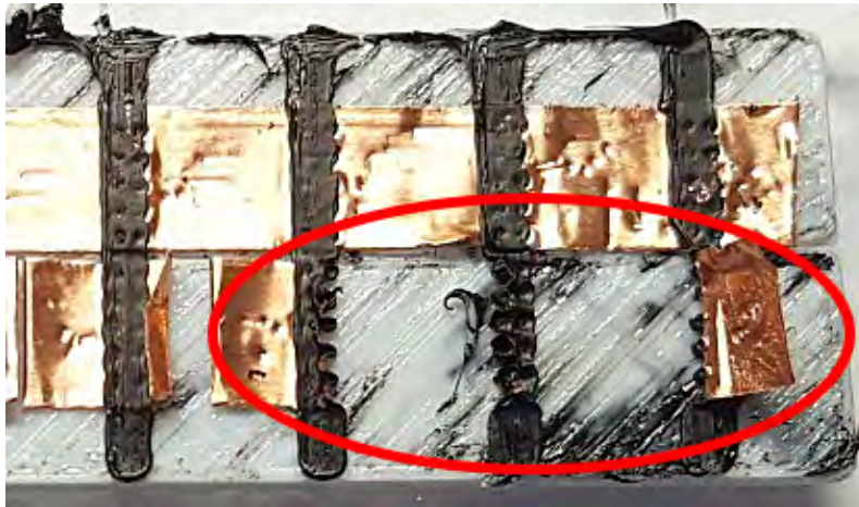
Figure 4.15: [NOTE: bed temperature 60°C] In the red circle you can see that the fusion between the ETPU and the Base layer (TPU) is so good that the tape just simply is pulled away from the connections so the 10 stakes stay in place and the tracksels are still attached.
