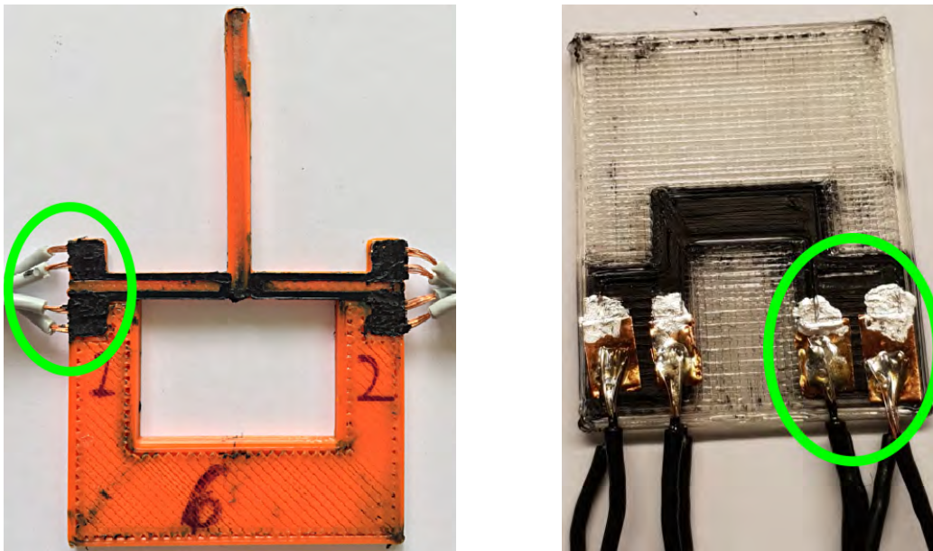
(a) Using a soldering iron to melt-in conductive wires into the conductive filament to establish a connection (green circle) [3]
