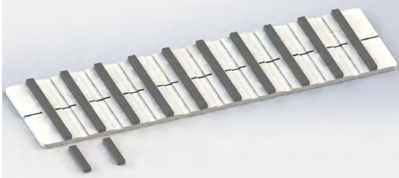
Figure 4.4: latest iteration of CAD model used to do the 10 sample test prints, model is both for ETPU and EPLA suitable. The black stripes are the printed conductive polymer traxels, that are printed on a white non-conductive base layer
