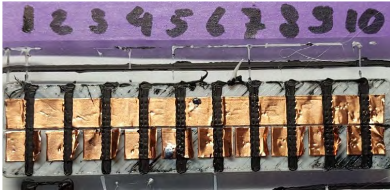
Figure 4.8: 10 ETPU tracks (black) printed over the punched holes in the copper tape connecting to a NinjaFlex base layer (white)
