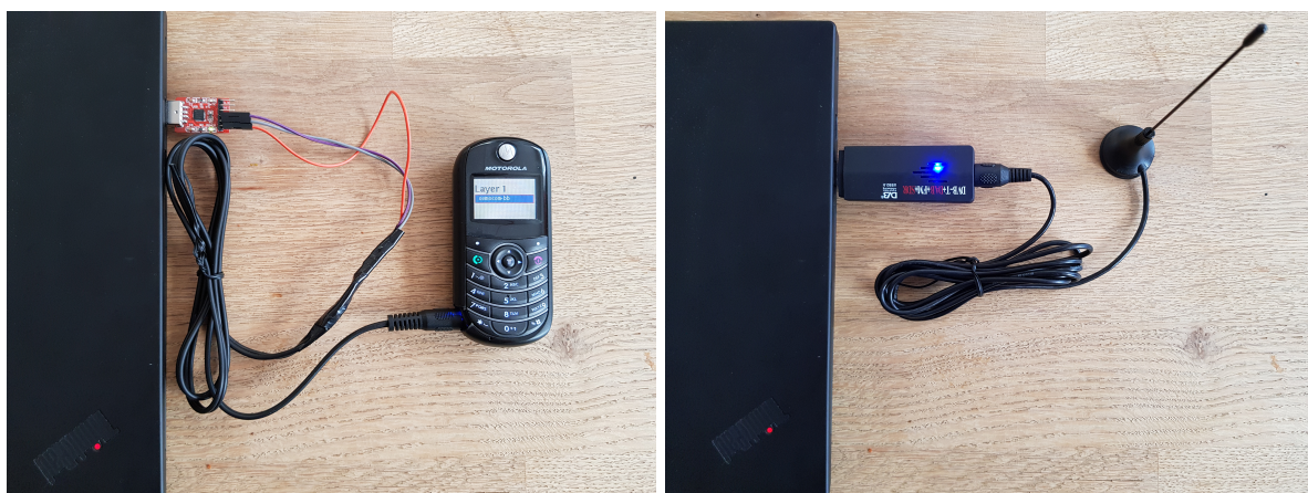
(a) The Motorola C139 running the OsmocomBB (b) A DVB-T dongle equipped with the RealTek RTL2832U chipset.
