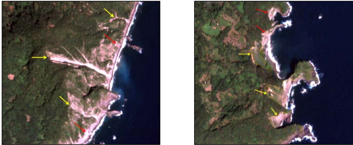
Figure 13. Examples of Landslide image interpretation in Dominica. A. The yellow arrows indicate Debris Slides (Left) and B. Rockslides (Right). The red arrows show areas of Rockfall.
