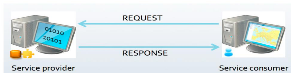
Figure 2-1 Web Service request-response mechanism
