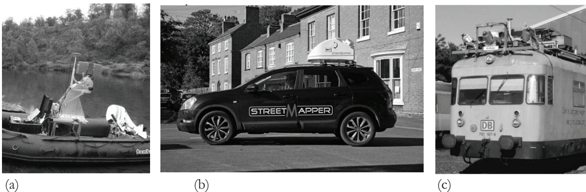
Figure 2-1: Mobile Laser Scanner platforms, (a) Boat (Alho et al., 2009) (b) Street Mapper Vehicle (c) Rail Mapper (Kremer & Grimm, 2012)
