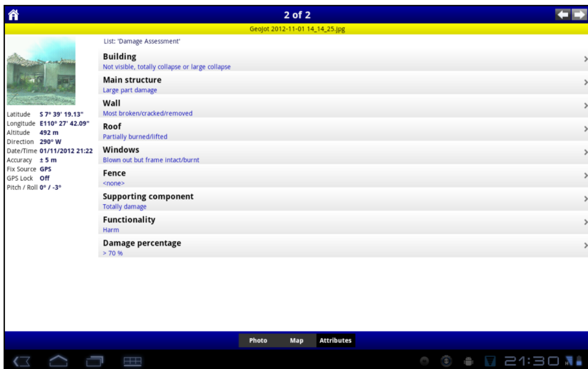
Figure 50. Building damage interpretation in Geojot
