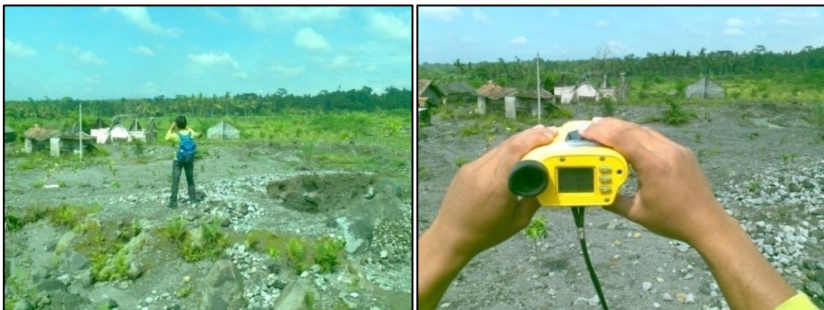
Figure 59. Measuring the distance between camera position and the object photographed with Laser Distance Meter (Laser Ace 300)
