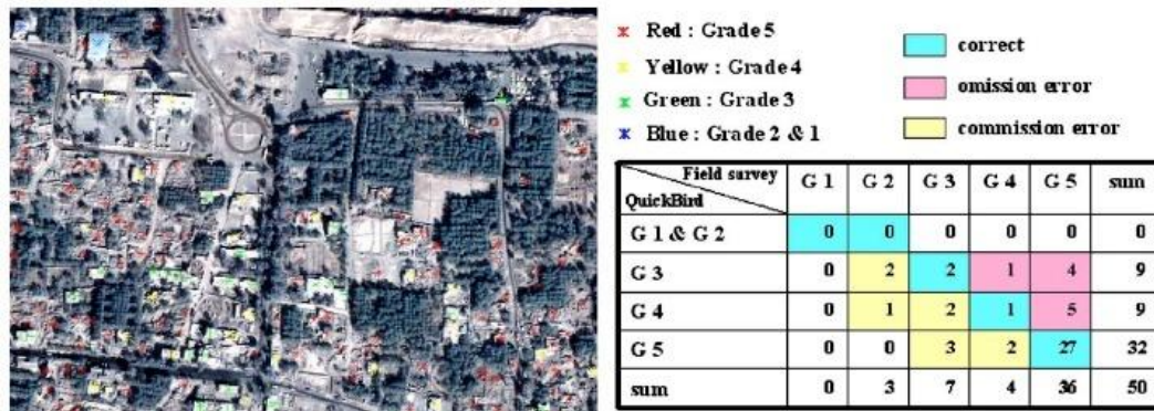
Figure 13. Accuracy assessment of the damage interpretation (Hisada et al (2005) in Yamazaki et al, 2005)
