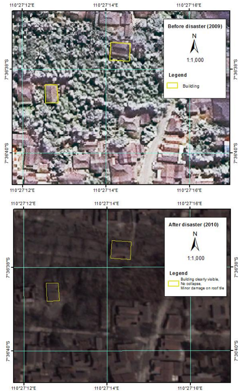
Figure 43. Building with criteria clearly visible/building still stands, no collapse, and minor damage on roof tile
