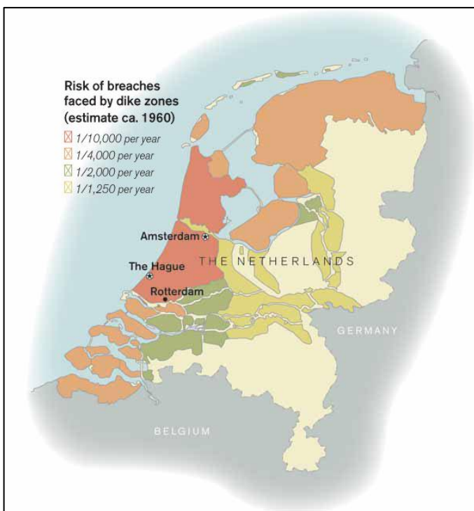
Figure 13 Map of Netherlands showing risk of breaches faced by dike zones (Source: Unknown)
