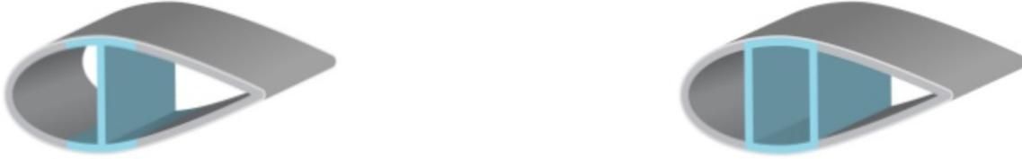
Figure 3: I-Spar (left) and box spar (right)
