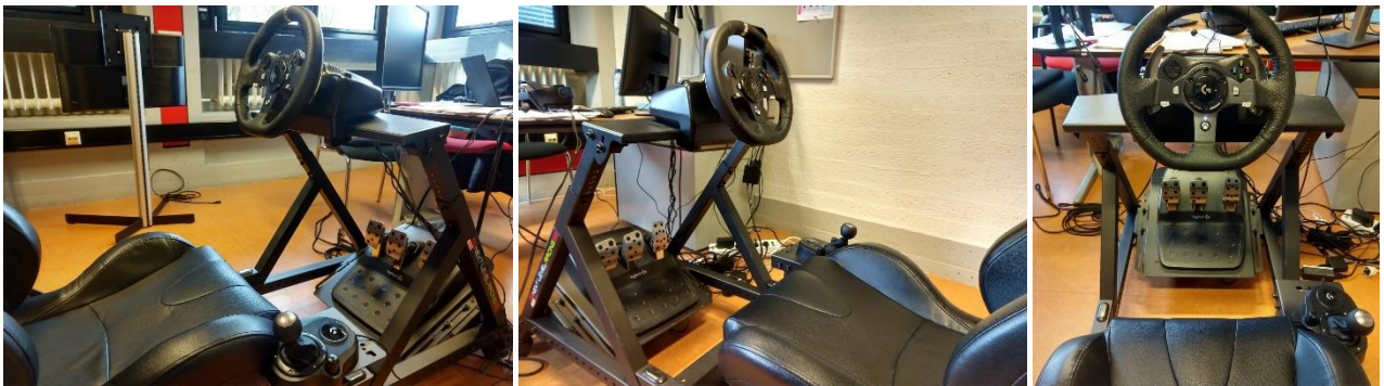
Figure 3. Driving simulator set-up. Participants could accelerate and brake by pressing the pedals and could manoeuvre by turning the steering wheel. The gear stick was not used.
