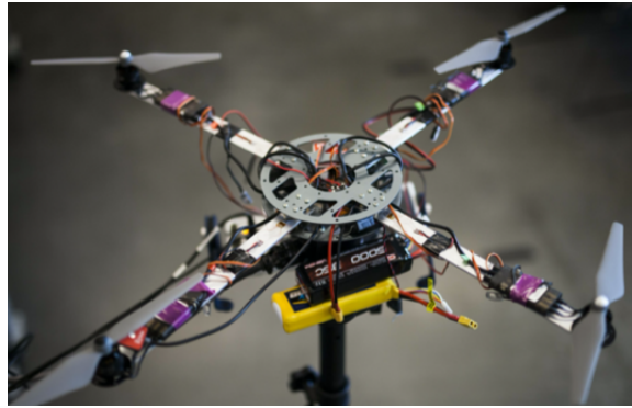
Figure 2.8: Quadcopter frame mounted onto a test stand comprising of load cells [7]
