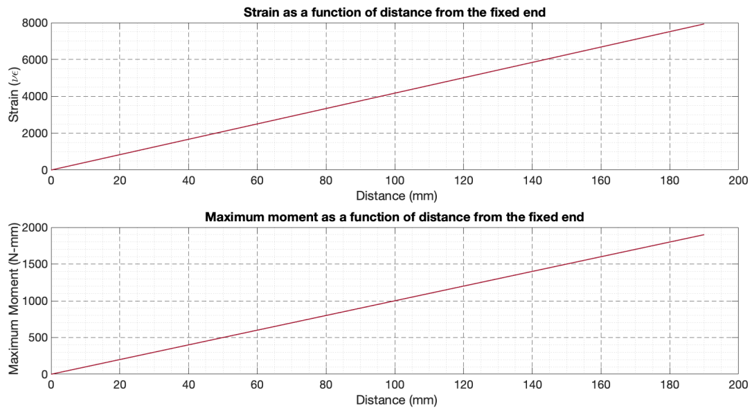
Figure 5.10: Strain and maximum moment on a cantilever as a function of distance from the fixed support
