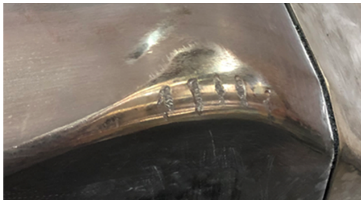
Figure 7.22: Severe galling on Side Member (white box) [64].
